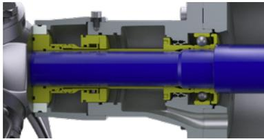
Single mechanical seal with flush SMS (FE)
